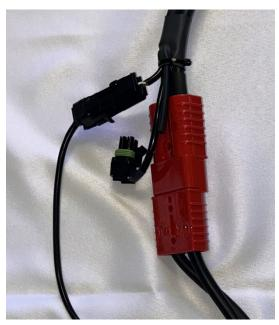
Connect the smaller cable from the Cold Switch to the matching connector from the ReadyWelder cable assembly.
