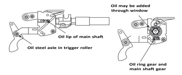
NOTE: Do not get oil on surface of plastic roller and main shaft. Use silicon oil on gears and shafts. Oil all parts sparingly with a toothpick or cotton swab.
