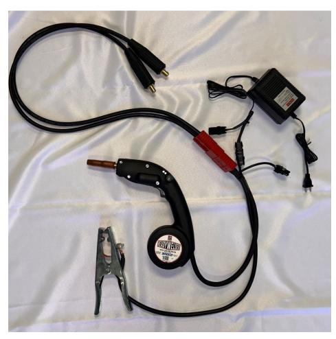
To connect the ReadyWelder to an external welding power source replace the battery clamp cable with the welder adapter cable that has the Dinse connectors. These connectors will mate with most welders. You may need to reverse polarity depending on whether you are doing straight connections or reverse connections.
