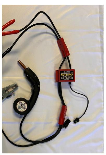
To install the Cold Switch disconnect the battery cable assembly from the ReadyWelder gun cable (large red connector).
