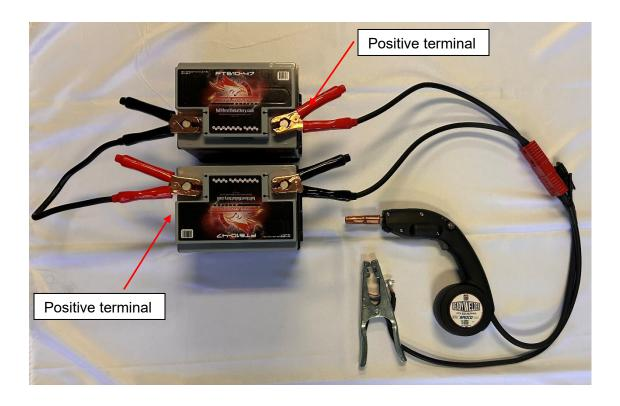
The ReadyWelder is configured to be in the straight polarity configuration when connected as in the figure above. When connected in this manner the green LED light on the ReadyWelder will illuminate. The welder will be ready to use with flux core wire which will be used in most remote applications.
