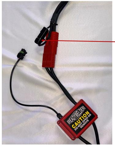
Locate the small data cable connectors coming from the ReadyWelder cable assembly.
